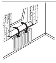
Danfoss Eco<sup>™</sup> features an Open-window function, which closes the valve if the room temperature is falling dramatically, thus reducing the heat loss. The heat is turned off for up to 30 minutes, before Danfoss Eco<sup>™</sup> returns to its original settings. When Open-window has been activated, the function is quarantined for 45 minutes.
